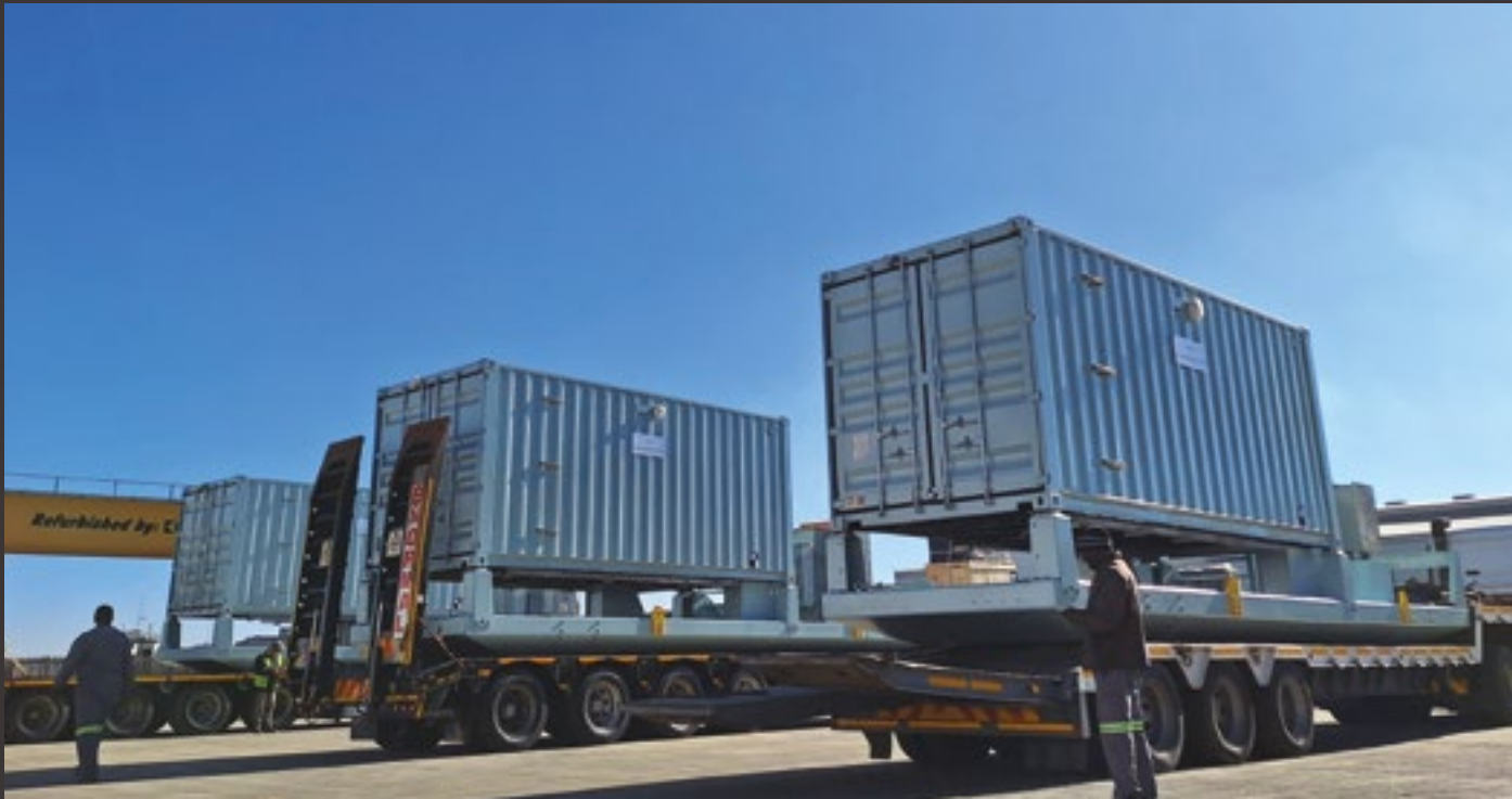
Fully welded laser-cut skid with containerised MCC, RMU, and transformer. Designed for crane lifting, easy on-site manoeuvring, and shipment as a fully assembled unit. MCC skids prepared for delivery to Kenmare Mine, Mozambique.
