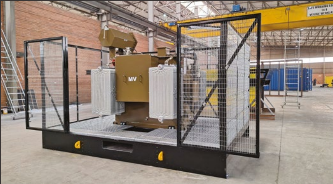
Heavy-duty 16m x 5m galvanised steel skid platform with banded grating and C5M marine-grade coating for corrosion resistance. Includes a 4,000 L polyurethane-lined integrated sump for secure high-voltage infrastructure containment.
